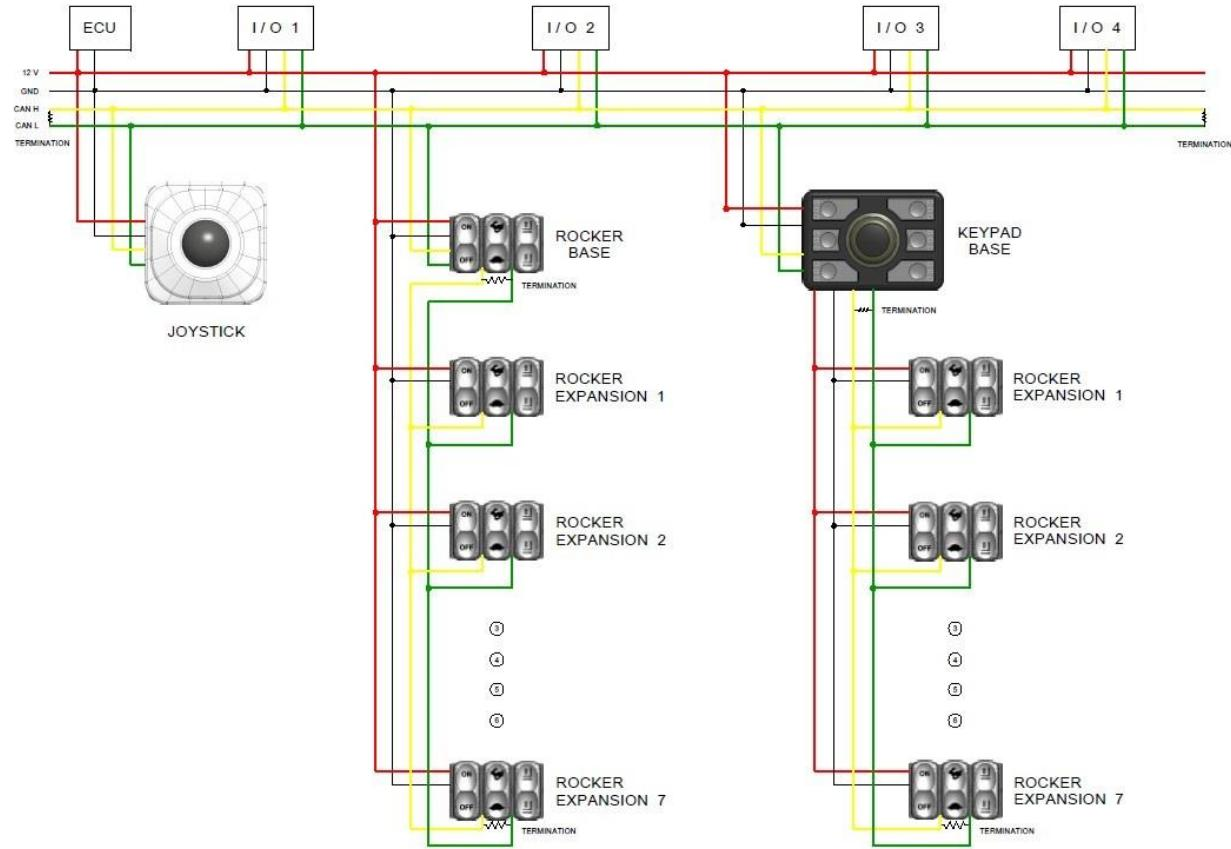
The rocker has an option to place a 120 Ohm CAN bus termination resistor within the module. Since most devices on the network do not have the termination, it is not installed as a default.
