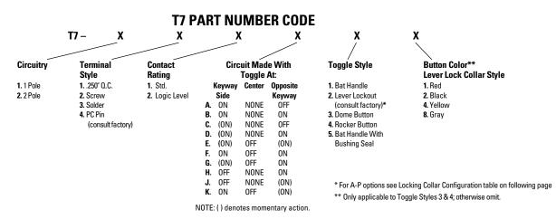
T7 Connector P/N C801765 (See Connector page in Hardware & Accessories section)
