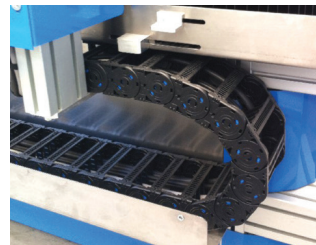
▶ ST 072N Application: Nylon Cloth cutting machine Location: Italy Remark: Stroke 2,5 meters
