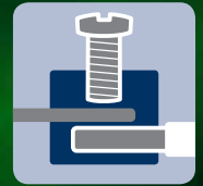
Screw connection system
