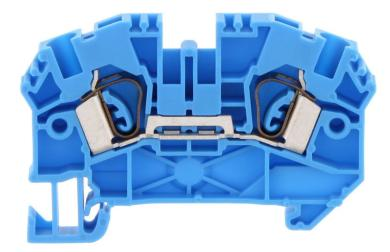
Feed-through terminal, Tension-spring connection, Mounting type: Mounting rail TS 35/7.5, Rated cross-section: 4 mm<sup>2</sup>, Width: 6.1 mm, Colour: Blue
