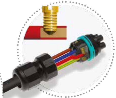
EN61984 certified piercing screw connector for flexible cables from 0.5 to 1.5 mm 2 (17.5A)
