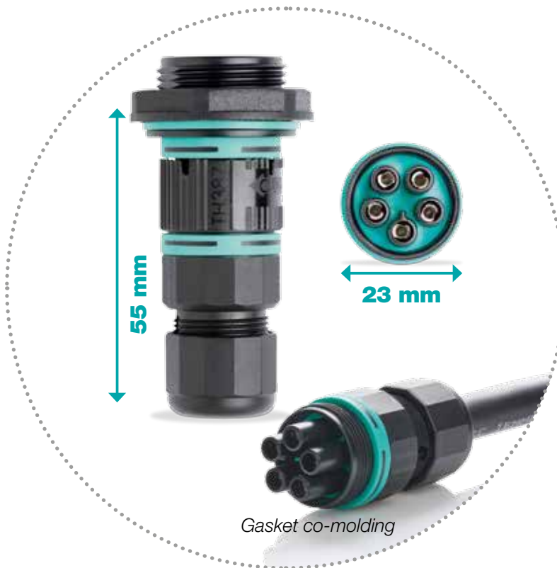
EN61984 certified piercing screw connector for flexible cables from 0.5 to 1.5 mm 2 (17.5A)
