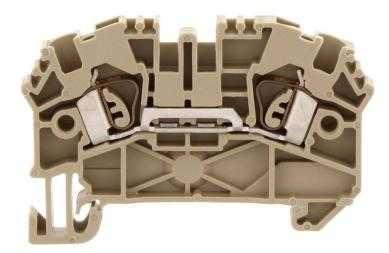
Feed-through terminal, Tension-spring connection, Mounting type: Mounting rail TS 35/7.5, Rated cross-section: 2.5 mm<sup>2</sup>, Width: 5.1 mm, Colour: Beige
