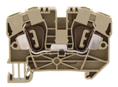
Feed-through terminal, Tension-spring connection, Mounting type: Mounting rail TS 35/7.5, Rated cross-section: 6 mm², Width: 8.1 mm, Colour: Beige
