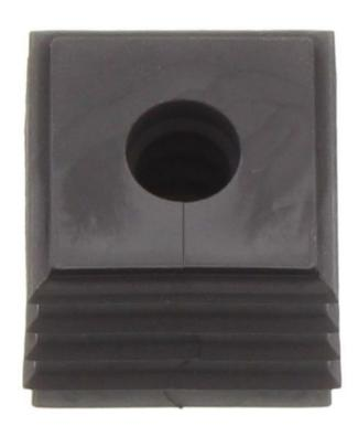
Seal, Mounting type: Plug in, Length x width: 20.3 mm, Max. cable diameter: 8 mm, IP 66, Colour: Black
