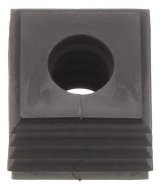
Seal, Mounting type: Plug in, Length x width: 20.3 mm, Max. cable diameter: 10 mm, IP 66, Colour: Black
