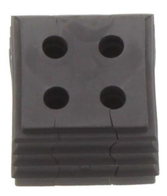
Seal, Mounting type: Plug in, Length x width: 20.3 mm, Max. cable diameter: 4 mm, IP 66, Colour: Black
