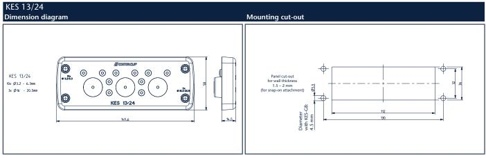
Torque for the frame's mounting screw: 2.5 - 3 Nm
