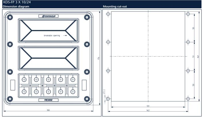
Torque for the frame's mounting screw: 3 Nm
