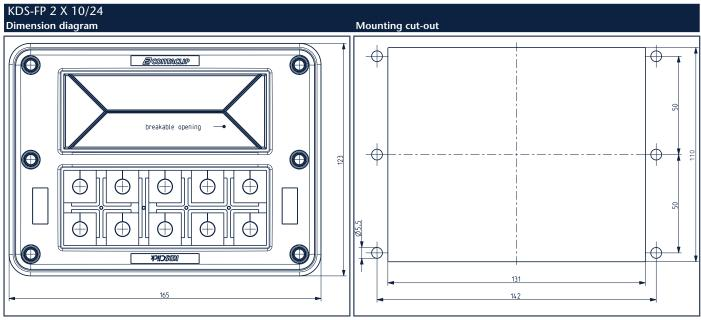
Torque for the frame's mounting screw: 3 Nm
