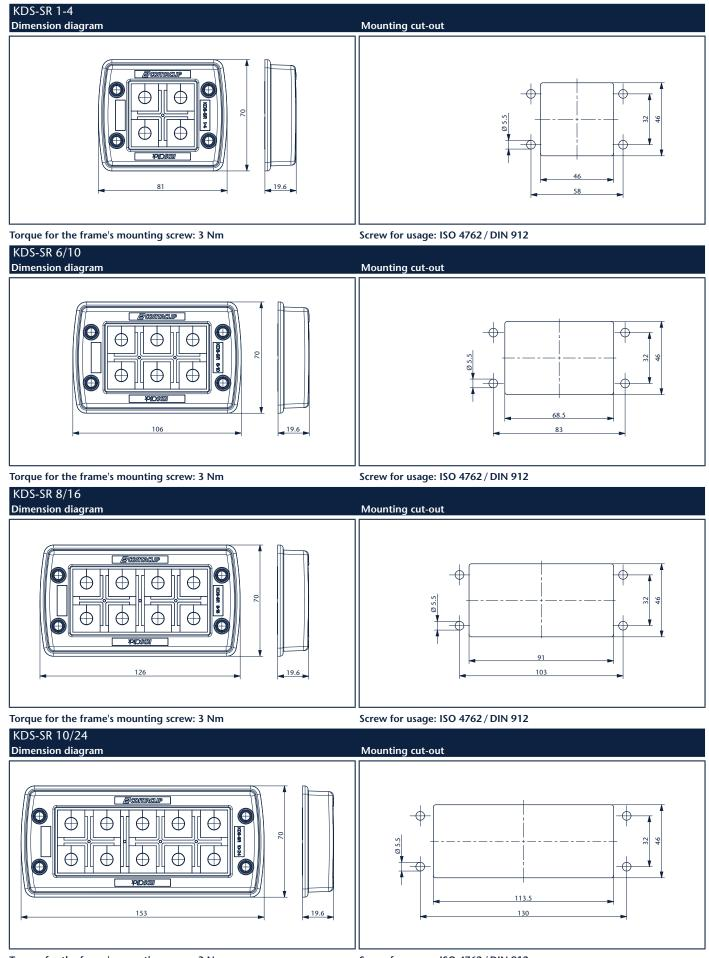
Torque for the frame's mounting screw: 3 Nm
