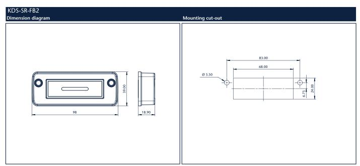
Torque for the frame's mounting screw: 3 Nm
