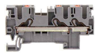
Feed-through terminal, Push-in connection, Mounting type: Mounting rail TS 35/7.5, Rated cross-section: 4 mm², Width: 6.1 mm, Colour: Grey
