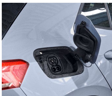
With vehicle charging inlet uncovered: IP6K6K/IP6K9K
