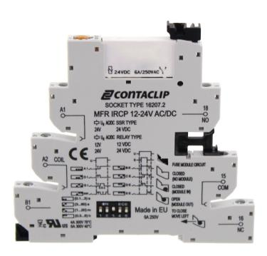
Multifunction timing relay module, Interface Relay Compact (IRC) complete, Consisting of base MFR-IRCP with Screw connection and Plug-in miniature relay PRC with power contact, Mounting type: TS 35, 1 Changeover contact, Input voltage: 12 VAC / DC
