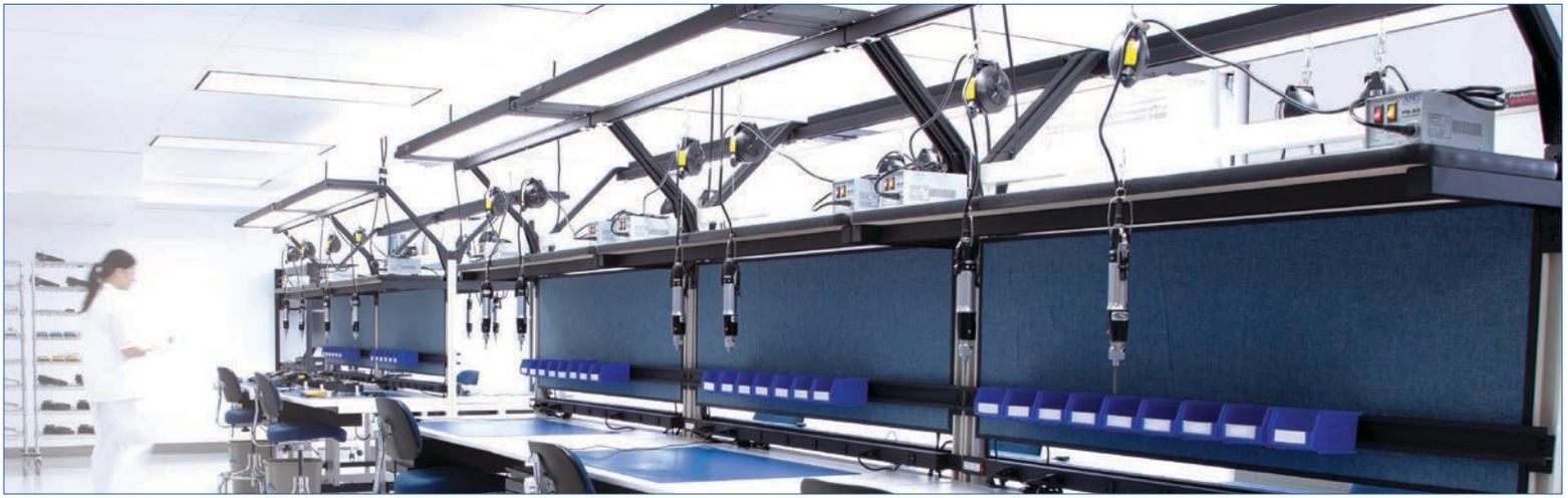
Every medical-grade foot control we manufacture is built in our Medical White Room, which features ESD Safe Construction for handling electronics, such as anti-static pads, grounded chairs, and grounding bracelets for technicians.
