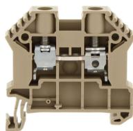
Feed-through terminal, Screw connection, Mounting type: Mounting rail TS 35/7.5, Rated cross-section: 10 mm<sup>2</sup>, Width: 8 mm, Colour: Beige
