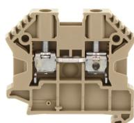
Feed-through terminal, Screw connection, Mounting type: Mounting rail TS 35/7.5, Rated cross-section: 2.5 mm<sup>2</sup>, Width: 5 mm, Colour: Beige
