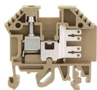
Feed-through terminal, Faston Spade connection / screw connection, Mounting type: Mounting rail TS 35/7.5 and TS 32, Rated cross-section: 2.5 mm<sup>2</sup>, Width: 6 mm, Colour: Beige
