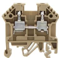
Feed-through terminal, Screw connection, Mounting type: Mounting rail TS 35/7.5 and TS 32, Rated cross-section: 4 mm<sup>2</sup>, Width: 6 mm, Colour: Beige
