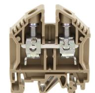
Ex feed-through terminal ATEX-certified, Screw connection, Mounting type: Mounting rail TS 35/7.5 and TS 32, Rated cross-section: 16 mm<sup>2</sup>, Width: 12 mm, Colour: Beige
