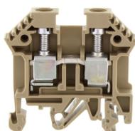
Ex feed-through terminal ATEX-certified, Screw connection, Mounting type: Mounting rail TS 35/7.5 and TS 32, Rated cross-section: 10 mm<sup>2</sup>, Width: 8 mm, Colour: Beige
