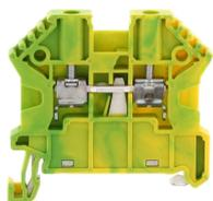
Protective earth terminal, Screw connection, Mounting type: Mounting rail TS 35/7.5, Rated cross-section: 2.5 mm<sup>2</sup>, Width: 5 mm, Colour: Green-yellow
