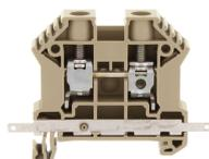
Feed-through terminal, Screw connection, Mounting type: Mounting rail TS 35/7.5, Rated cross-section: 16 mm<sup>2</sup>, Width: 10 mm, Colour: Beige
