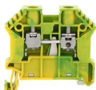
Protective earth terminal, Screw connection, Mounting type: Mounting rail TS 35/7.5, Rated cross-section: 10 mm<sup>2</sup>, Width: 8 mm, Colour: Green-yellow
