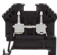
Feed-through terminal, Screw connection, Mounting type: Mounting rail TS 35/7.5, Rated cross-section: 4 mm<sup>2</sup>, Width: 6 mm, Colour: Black
