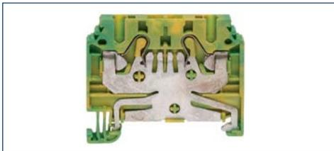
A protective-earth (PE) terminal block is a device with one or more clamping points used to connect round conductors (PE/PEN wires). The PE terminal contacts the metal DIN rail via the PE foot using either a screw attachment or by simply snapping on the terminal block to the rail (using an internal-spring PE foot).
