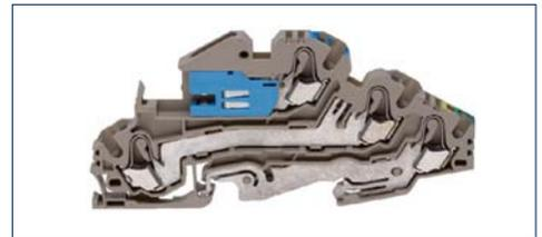
A multi-level terminal block is a device that features at least two busbar levels. Four or more terminal points are available to connect round conductors. A variety of combination options are possible: L/PE, L/L, L/N, N/N, N/PE or L/N/PE, L/L/N, N/N/PE, etc.
