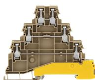
Motor-connection terminal, Screw connection, Mounting type: Mounting rail TS 35/7.5, Rated cross-section: 2.5 mm<sup>2</sup>, Width: 6 mm, Colour: Beige
