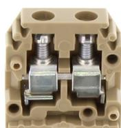
Feed-through terminal for direct mount, Screw connection, Mounting type: Mounting surface, Rated cross-section: 4 mm<sup>2</sup>, Width: 6 mm, Colour: Beige
