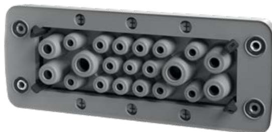
Using the latching clips, the **KES-GB** latches onto the outside of the housing wall. It is then screwed on from the inside, through the housing wall, using the integrated threaded bushes.
