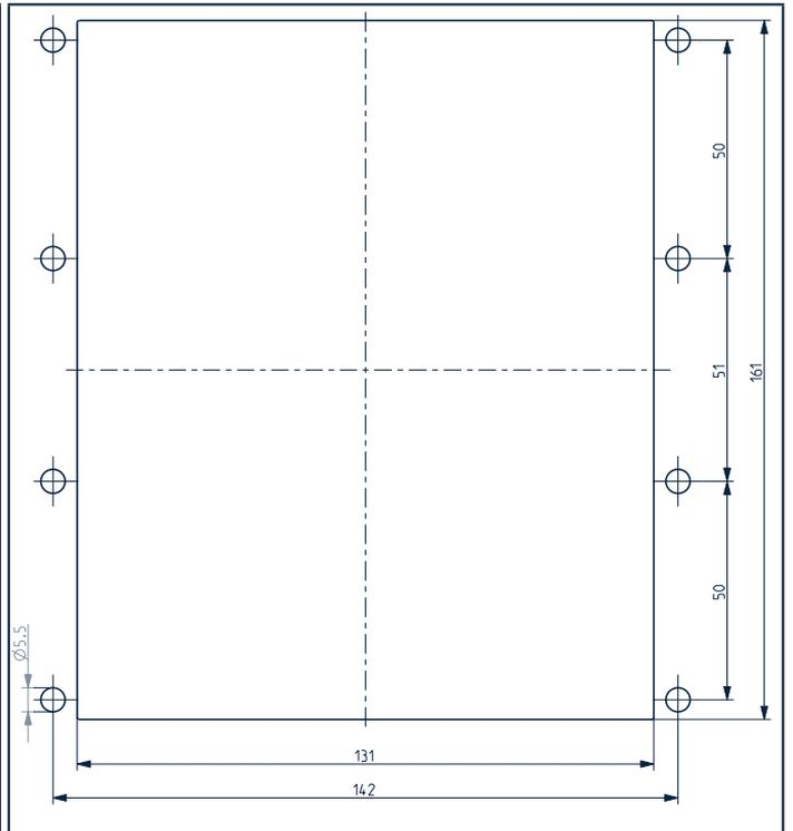
Screw for usage: ISO 4762 / DIN 912
