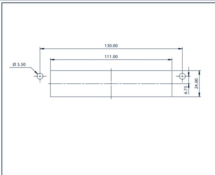
Screw for usage: ISO 4762 / DIN 912
