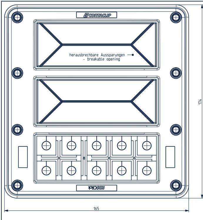
Torque for the frame's mounting screw: 3 Nm
