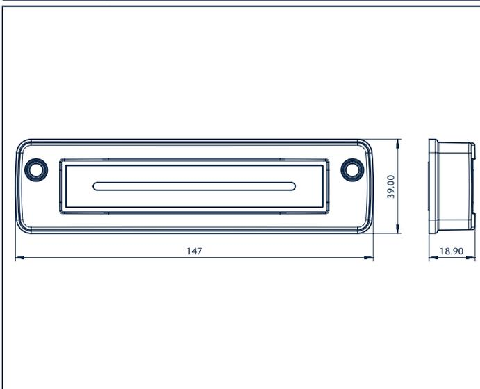
Torque for the frame's mounting screw: 3 Nm
