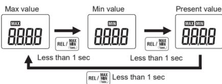
\* To activate MAX/MIN function, REL function should be disabled.
