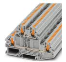
Double-level terminal block, nom. voltage: 800 V, nominal current: 22 A, connection method: Push-in connection, 1st and 2nd level, Rated cross section:  $2.5~\text{mm}^2$ , cross section:  $0.14~\text{mm}^2$  -  $4~\text{mm}^2$ , mounting type: NS 35/7,5, NS 35/15, color: gray
