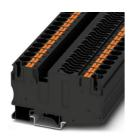
Fuse modular terminal block, fuse type: Blade, fuse type: C, nom. voltage: 400 V, nominal current: 25 A, connection method: Push-in connection, Rated cross section: 10 mm<sup>2</sup>, cross section:  $0.5 \text{ mm}^2$ - 16 mm<sup>2</sup>, mounting type: NS 35/7,5, NS 35/15, color: black
