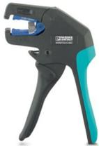
Stripping tool, for cables and conductors (especially for cables protected against short circuits and ground leakages) 1.5 - 6 mm<sup>2</sup>, self-adjusting, stripping length of up to 18 mm, cutting capacity of up to 10 mm<sup>2</sup> stranded/1.5 mm<sup>2</sup> solid, replaceable stripping blade
