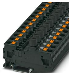
Fuse modular terminal block, fuse type: Glass / ceramics / ..., fuse type: G / 5 x 20, nom. voltage: 250 V, nominal current: 10 A, connection method: Push-in connection, Rated cross section: 6 mm<sup>2</sup>, cross section: 0.5 mm<sup>2</sup>- 10 mm<sup>2</sup>, mounting type: NS 35/7,5, NS 35/15, color: black
