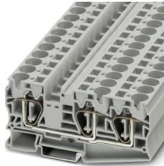
Feed-through terminal block, nom. voltage: 1000 V, nominal current: 76 A, number of connections: 3, connection method: Spring-cage connection, Rated cross section: 16 mm<sup>2</sup>, cross section: 0.2 mm<sup>2</sup> - 25 mm<sup>2</sup>, mounting type: NS 35/15, NS 35/7,5, color: gray
