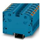
High-current terminal block, nom. voltage: 1000 V, nominal current: 125 A, number of connections: 2, connection method: PowerTurn connection, Rated cross section: 35 mm<sup>2</sup>, cross section: 2.5 mm<sup>2</sup> - 35 mm<sup>2</sup>, mounting type: NS 35/15, color: blue
