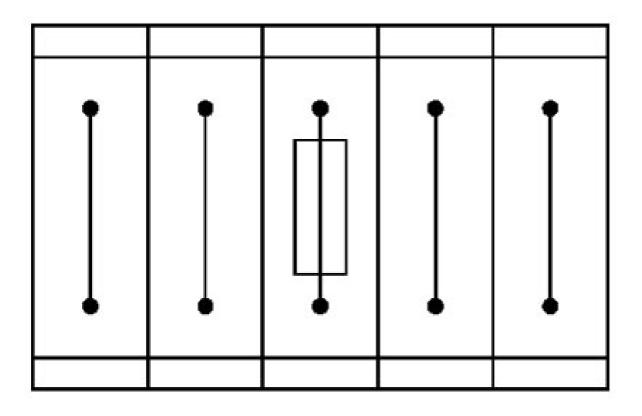
Fuse terminal block in single arrangement,
