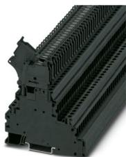
Fuse modular terminal block, fuse type: Glass / ceramics / ..., fuse type: G / 5 x 20, nom. voltage: 24 V, Thermal continuous current  $I_{th}$ : 28 A, connection method: Screw connection, Rated cross section: 4 mm<sup>2</sup>, cross section: 0.14 mm<sup>2</sup>- 6 mm<sup>2</sup>, connection method: Screw connection, Rated cross section: 4 mm<sup>2</sup>, cross section: 0.14 mm<sup>2</sup>- 6 mm<sup>2</sup>, mounting type: NS 35/7,5, NS 35/15, color: black
