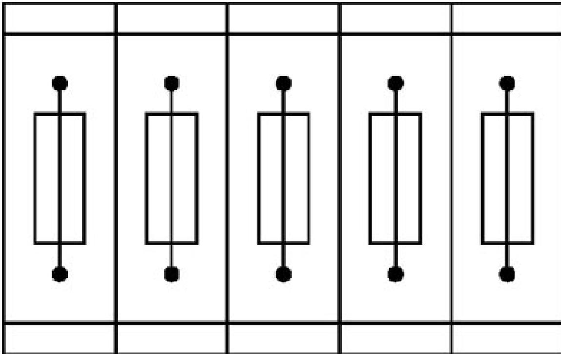
Fuse terminal blocks in interconnected arrangement,
