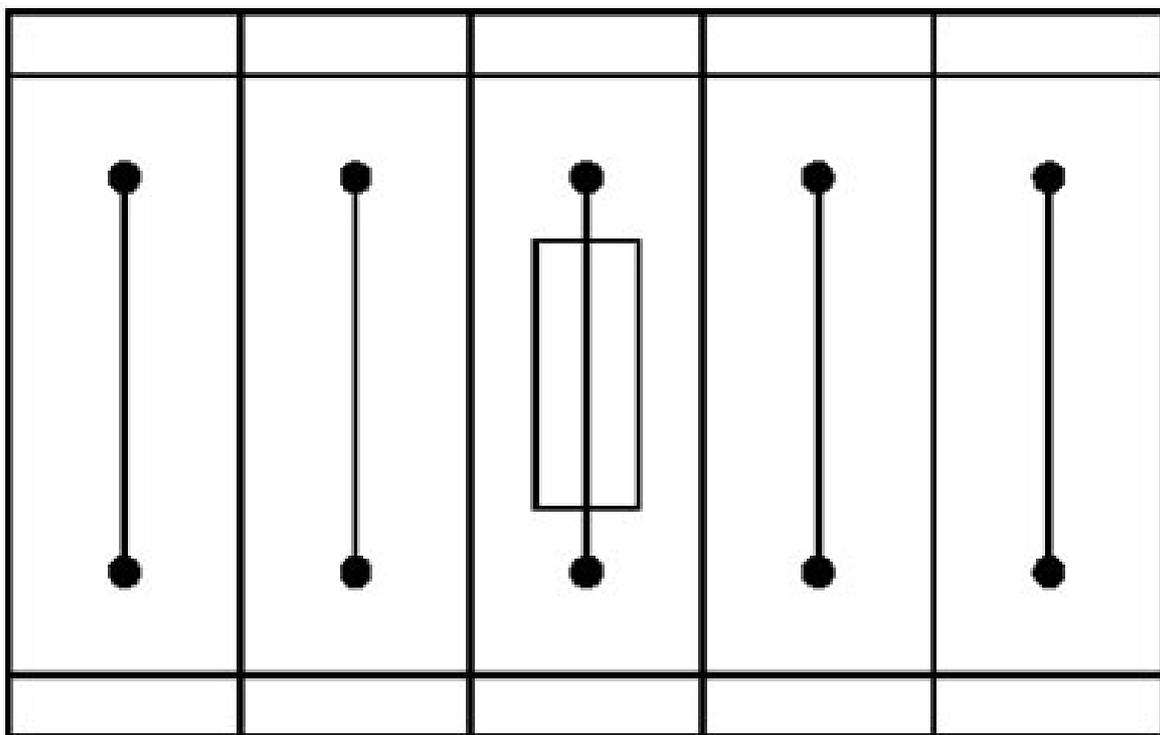
Fuse terminal block in single arrangement,
