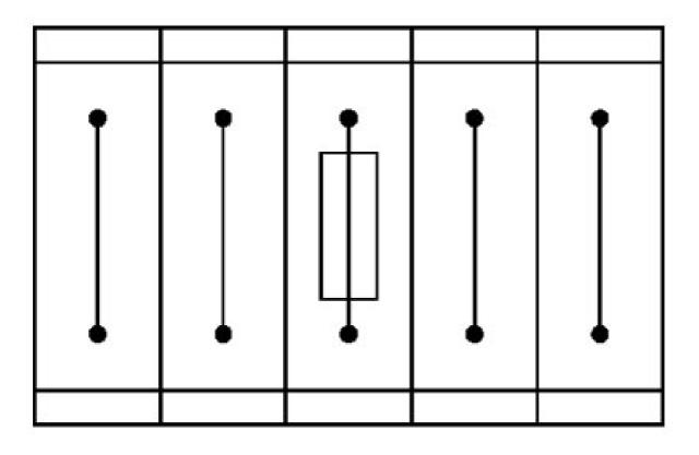
Fuse terminal block in single arrangement,
