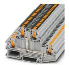
Double-level terminal block, nom. voltage: 800 V, nominal current: 22 A, connection method: Push-in connection, 1st and 2nd level, Rated cross section: 2.5 mm², cross section: 0.14 mm² - 4 mm², mounting type: NS 35/7,5, NS 35/15, color: gray
