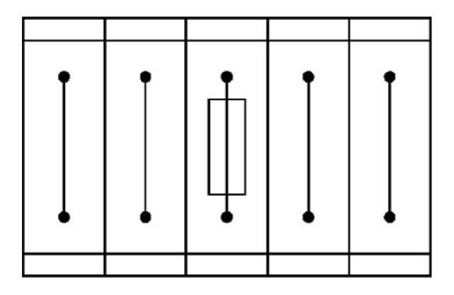
Fuse terminal block in single arrangement,
