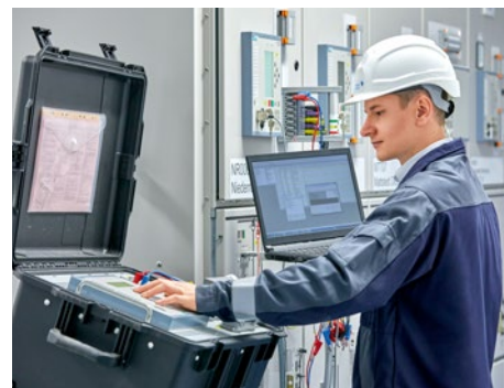
The FAME plug-in test systems enable easy testing even outside the control cabinet. This means that you can perform testing in the field of mains protection technology safely and in no time at all.
