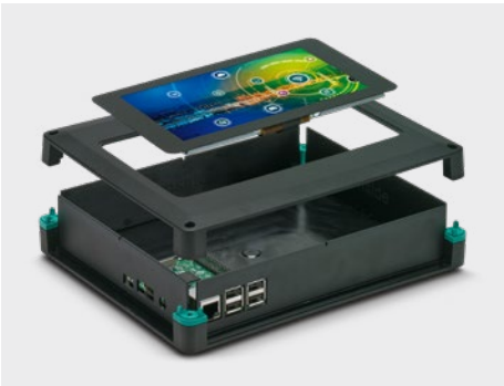
Easy integration of the Raspberry Pi touch display and increased functionality with more space available for individual circuits.
