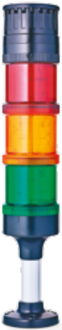
Order number: ECO70-Q31 Colours: red/orange/green Function: LED steady beacon, buzzer steady or pulsing tone Nominal voltage: 24 V AC/DC Type of mounting: Tube mounting (100 mm tube length)
