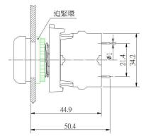
Dimensions with front facing Screw terminal contact block installation
