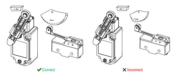
• Appropriate force must be imposed on the actuator by the cam or dog in both rotary operation and linear operation. If the dog touches the lever as shown below, the operating position will not be stable.
