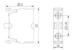
Adapter for front facing buckle contact blocks (A3)
