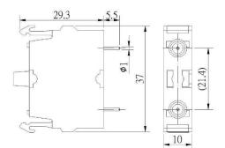
Contact Block (SB) -Screw terminal, Back facing (for M22 Box)
