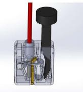
2. Insert wire securely. Once secure, release pin tool for clamp to engage with wire.
