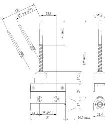
MN-5166 | OF MAX 120g RF MIN -PT MAX 25mm OT MIN 11mm DT MAX -
