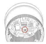
Located here (red circle) is the selector to switch between different modes of function.
