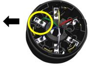
$\bigcirc$  DO NOT USE excessive force when installing wires.  $\bigcirc$  DO NOT USE non-compliant pin tools to install wires, doing so damages the unit.
