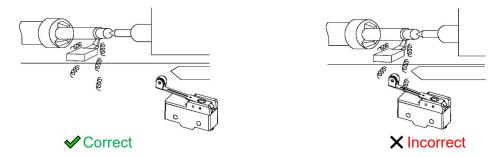
• Constantly subjecting a Switch to vibration or shock can result in wear, which can lead to contact interference with contacts, operation failure, reduced durability, and other problems. Excessive vibration or shock can lead to false contact operation or damage. Install Switches in locations not subject to shock and vibration and in orientations that will not produce resonance.
