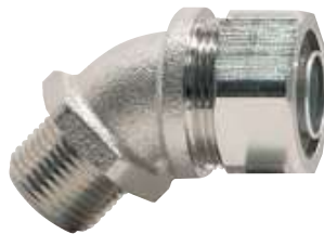
LC - 45 - B (IP66/67/68) External Male Thread 45 degree bend Multi part compression fitting with a nylon seal Available in Zinc Plated Steel, Nickel Plated Brass (B) and 316 Stainless Steel (SS)
