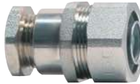
LC - SPS (IP66/67/68) Space Saver Multi part compression fitting with a nylon seal. Contains female threaded body component and a male threaded bush component , which minimises the amount of space taken up inside enclosures. Available in Brass (B)
