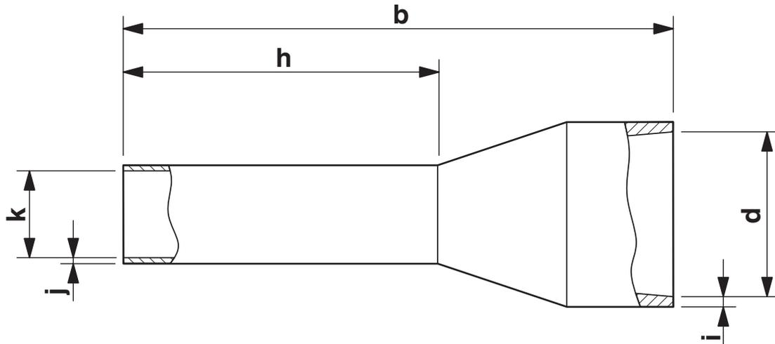
Sleeve length (b), length contact range (h), insulating collar inner dimension (d), sleeve diameter (k), insulating collar thickness (i), sleeve wall thickness (j)
