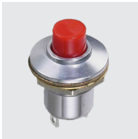
P3: Sealed, Momentary Action or Push-Pull
