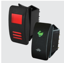
K5: Sealed, Illuminated with Legend Options, Single Pole Triple Throw
