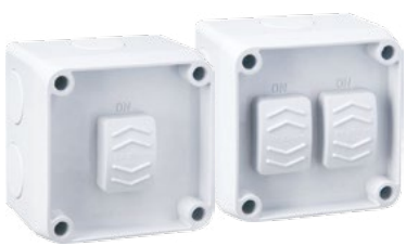
Dual 25mm screwed conduit entries top and bottom (up to 63 amp) allows four ways to surface wire the switch.
